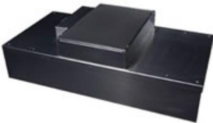
The MAC 10<sup>®</sup> IQ is the world's first smart Fan Filter Unit (FFU). With its microcomputer controlled electrically commutative (EC) motor, the MAC 10 IQ dynamically adjusts itself to maintain the set airflow, compensating for changes in static pressure, filter loading or other local conditions. Competitively priced, the MAC 10 IQ offers low sound, low energy consumption and a low profile, with high performance and built-in intelligent control.
